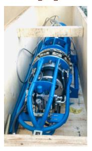
**Internal Pneumatic Pipe Line Up Clamp**
